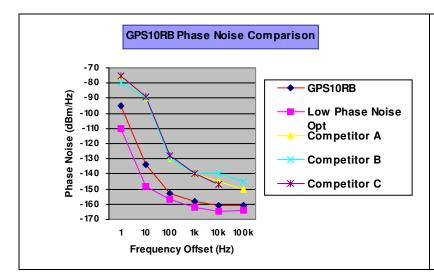
The graph to the left shows the GPS10RBN phase noise (red trace) compared with three competitors (Yellow, Purple and Blue traces). As can be seen the GPS10RBN has lower phase noise than its competitors.
